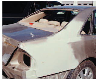
Collision WRAP for sitting vehicle in phases of repair.
